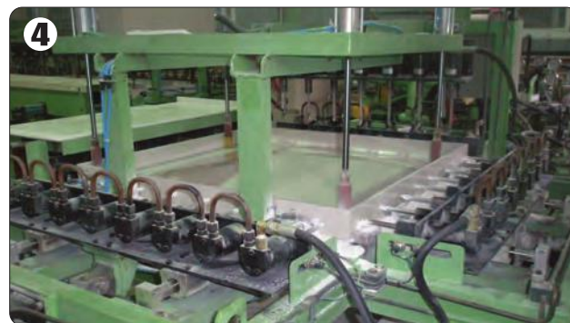
Drill on the GRP panel
